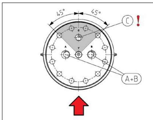
Figure 3. Motor orientation to the load direction.
